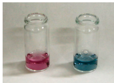
Fig. 6 Observed color change of a 0.25 mM aqueous solution of PyC8TOV (red, left) caused by the addition of 50 mM NaCl (blue, right).
